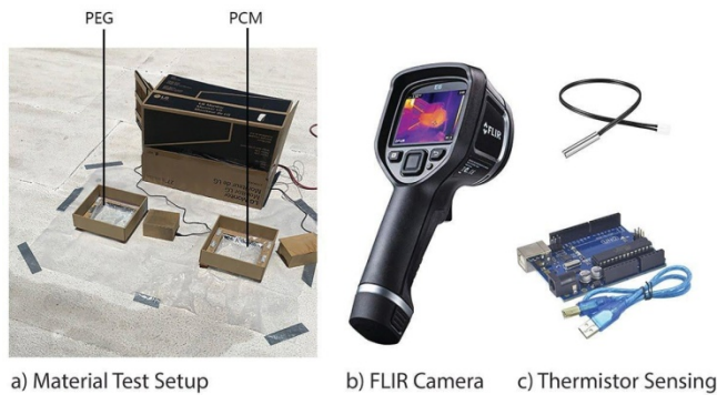
Figure 3. Material pilot test setup: a) Polyelectrolyte Gel (PEG) and Phase Change Material (PCM) testing modules; b) FLIR camera used for thermography images; and c) Thermistor sensing for material temperature data collection
