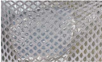
Figure 2. Hydrogel adhered to flexible mesh
