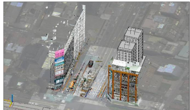
Figure 3. The overlapping of point clouds, new building design, and aerial photos
