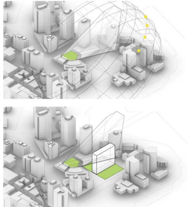
Figure 11. Trim the building to ensure solar rights
