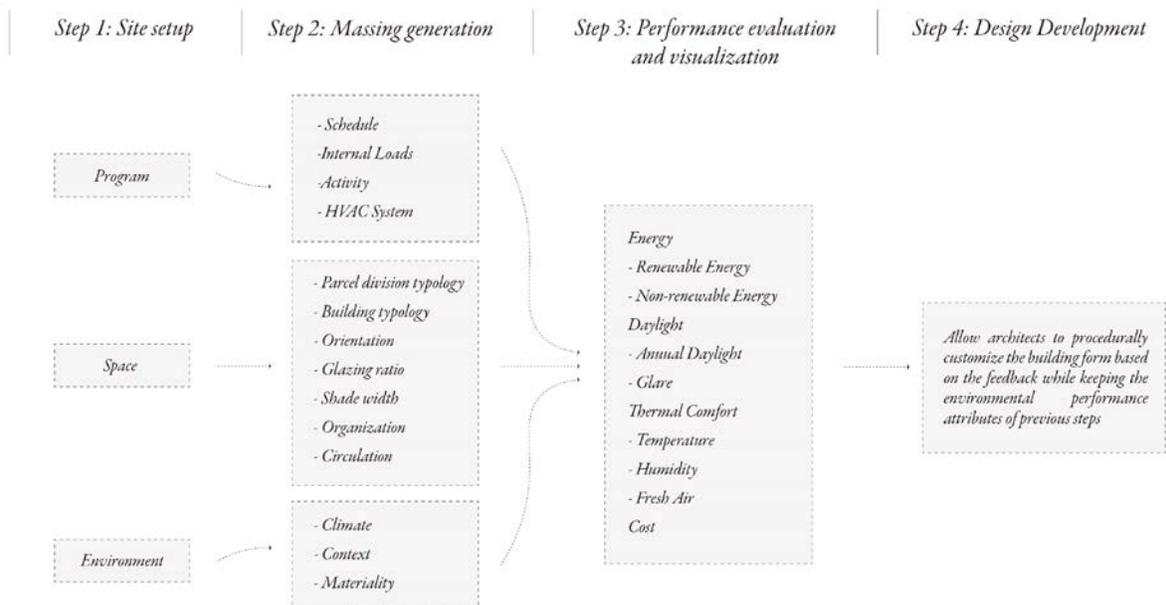
Figure 1. New workflow for high-performance building form design
