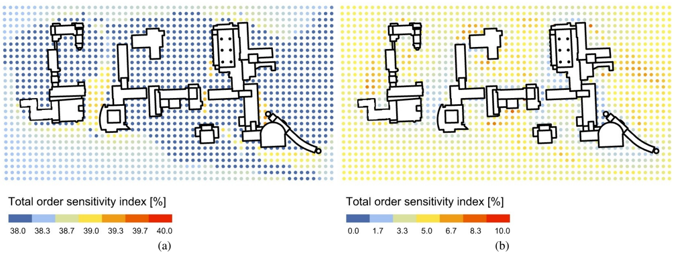
Figure 6. Spatially-resolved total sensitivity index for the (a) the wind velocity and (b) the mean radiant temperature.
