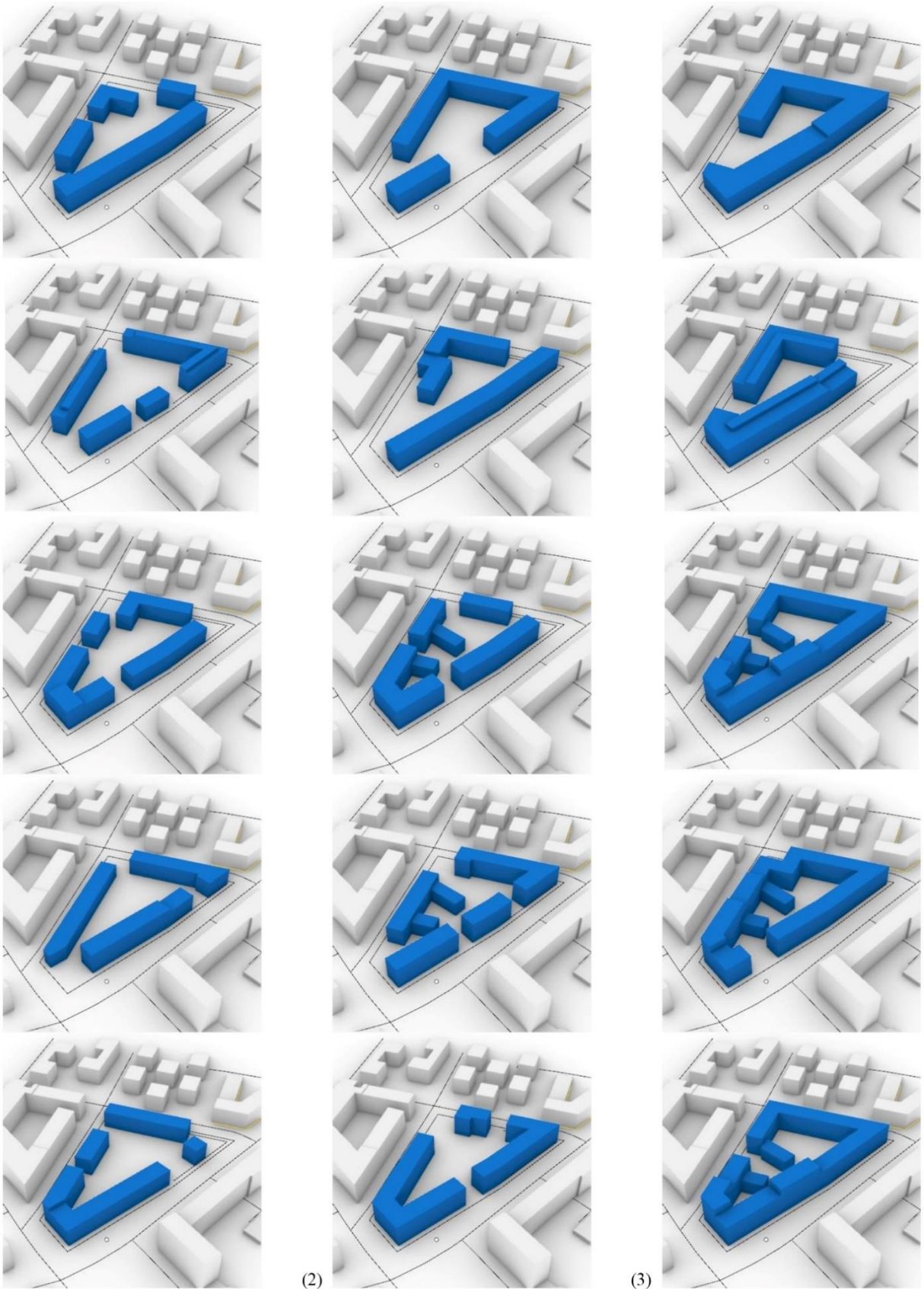
Figure 10. Examples of the designs for 3 sub-sets of the generation outputs: (1) FAR = 1.7 +/- 0.5; (2) FAR = 2.2 +/- 0.5; (3) FAR = 3.0 +/- 0.05.
