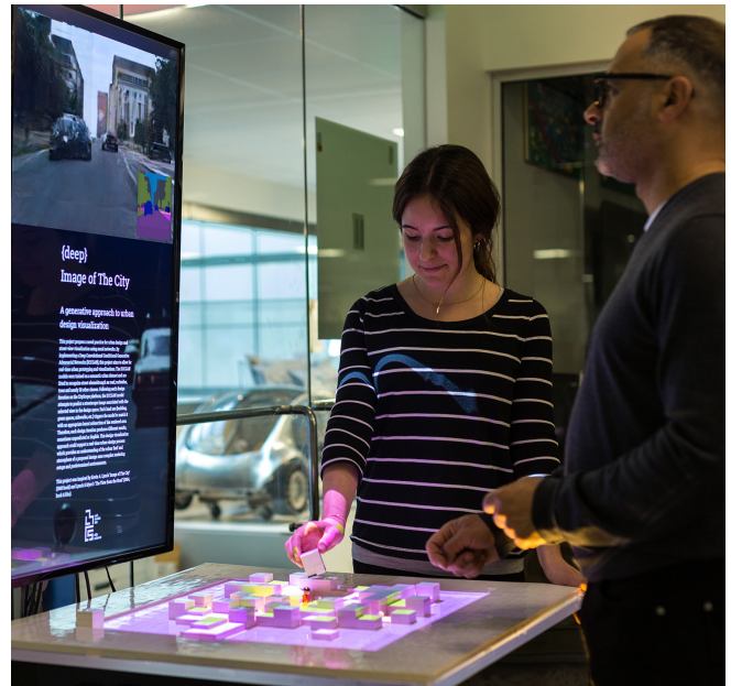
Figure 1. DeepScope TUI: Multiple users can simultaneously interact and discuss urban design iterations. The table-top is used as both the design space and a schematic urban top-view. The vertical monitor visualizes the DCGAN street view.
